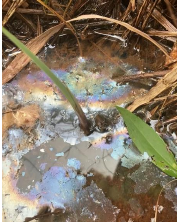
Figure 15. Photo showing rainbow sheen on the surface of groundwater-fed water. Note that the sheen can be broken apart unlike the sheen from oils. (Photo credit: Sally Jarosz, WDNR).
