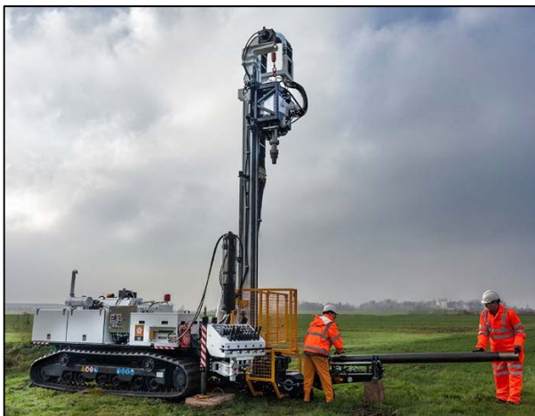
Photos 7 and 8 - Rotosonic drilling rig (left) (Boart Longyear) and examples of subsurface samples collected from Rotosonic drilling (right) (GeoDesign, Inc).
