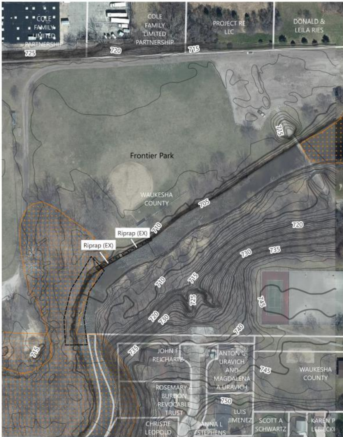
Figure 3.3 – Streambank stabilization locations within property.
