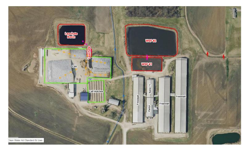
Site Overview Diagram (Main Dairy: orange lines =potential runoff flow patterns, blue lines = stormwater flow, pink lines = waste transfer system, yellow circles indicate water supply well locations)
