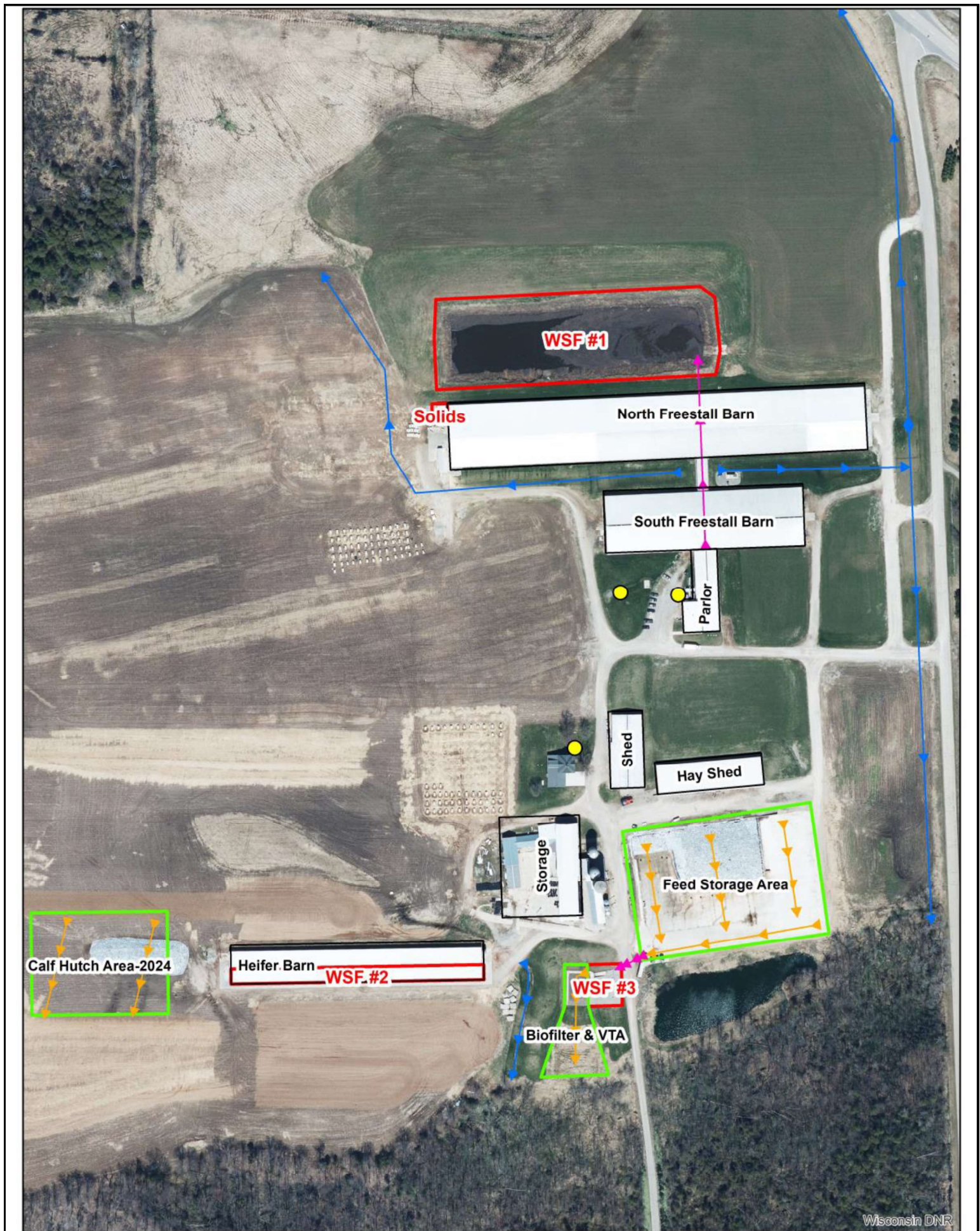
Site Overview Diagram (Tauchen Harmony Valley: orange lines = potential contaminated runoff, blue lines = stormwater flow, pink lines = waste transfer system, yellow circles = well locations)
