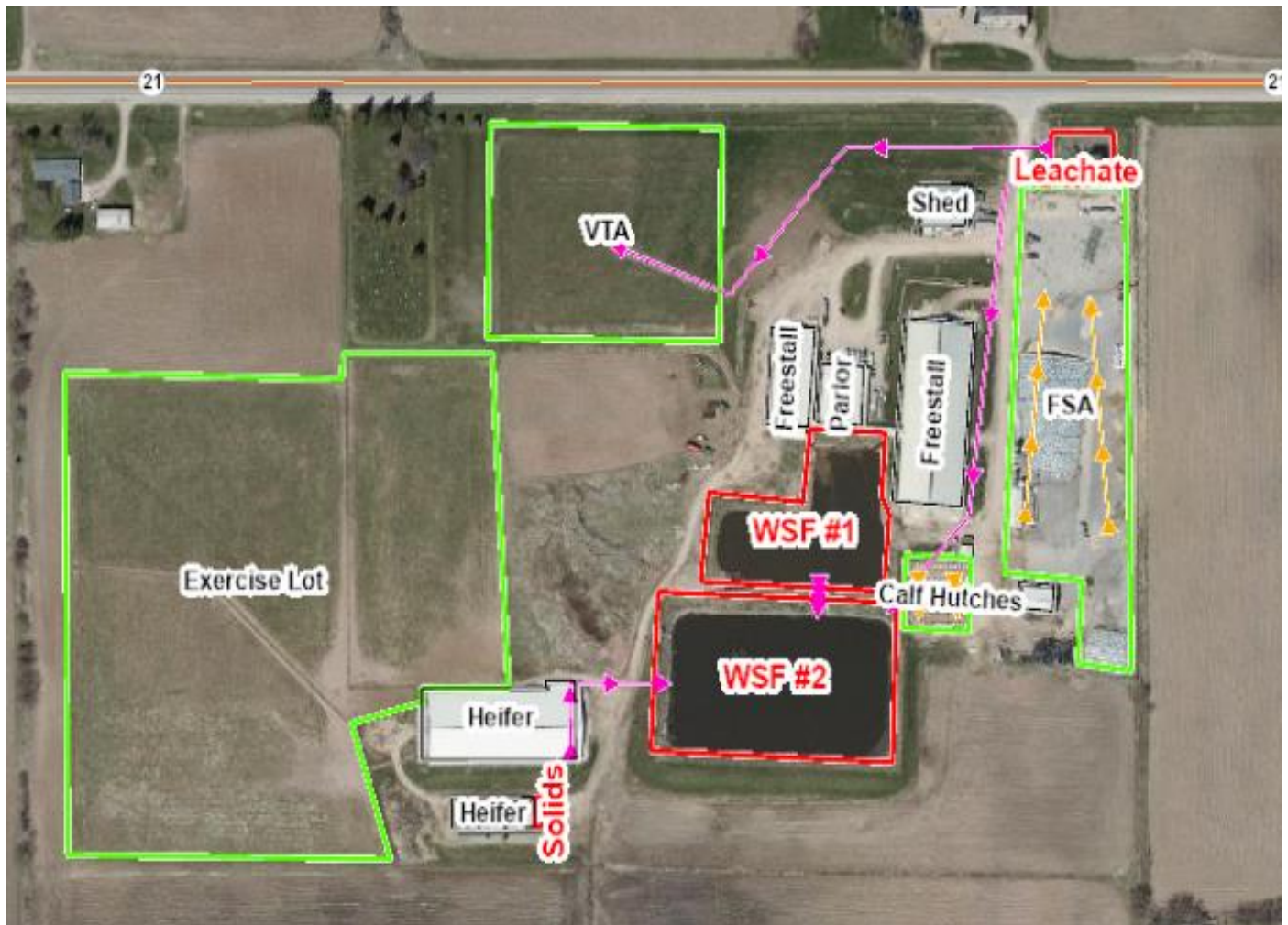
Figure 1. Aerial overview of Krentz Family Dairy Main Dairy site. Yellow arrows indicate approximate contaminated runoff flow paths, pink arrows indicate manure transfer systems.
