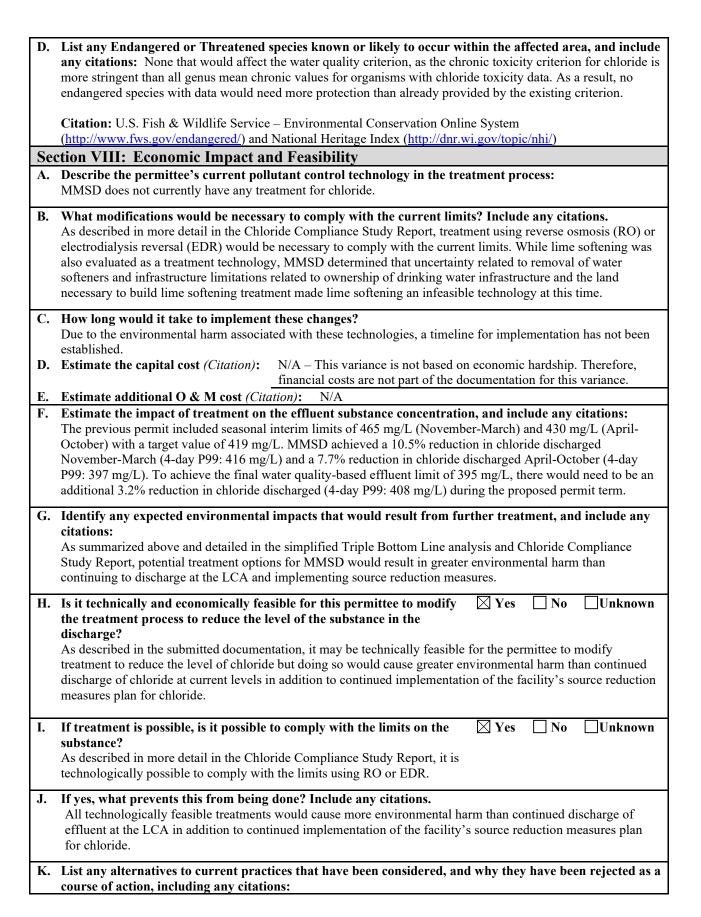
As described in the Chloride Compliance Study Report the following technologies were evaluated; lime softening, electrodialysis reversal (EDR), and reverse osmosis (RO). All were rejected as a course of action either due to uncertainty of compliance (lime softening) or greater amounts of environmental harm from installing treatment than continued discharge at LCA (EDR; RO) and continued implementation of the facility's source reduction measures plan for chloride.
