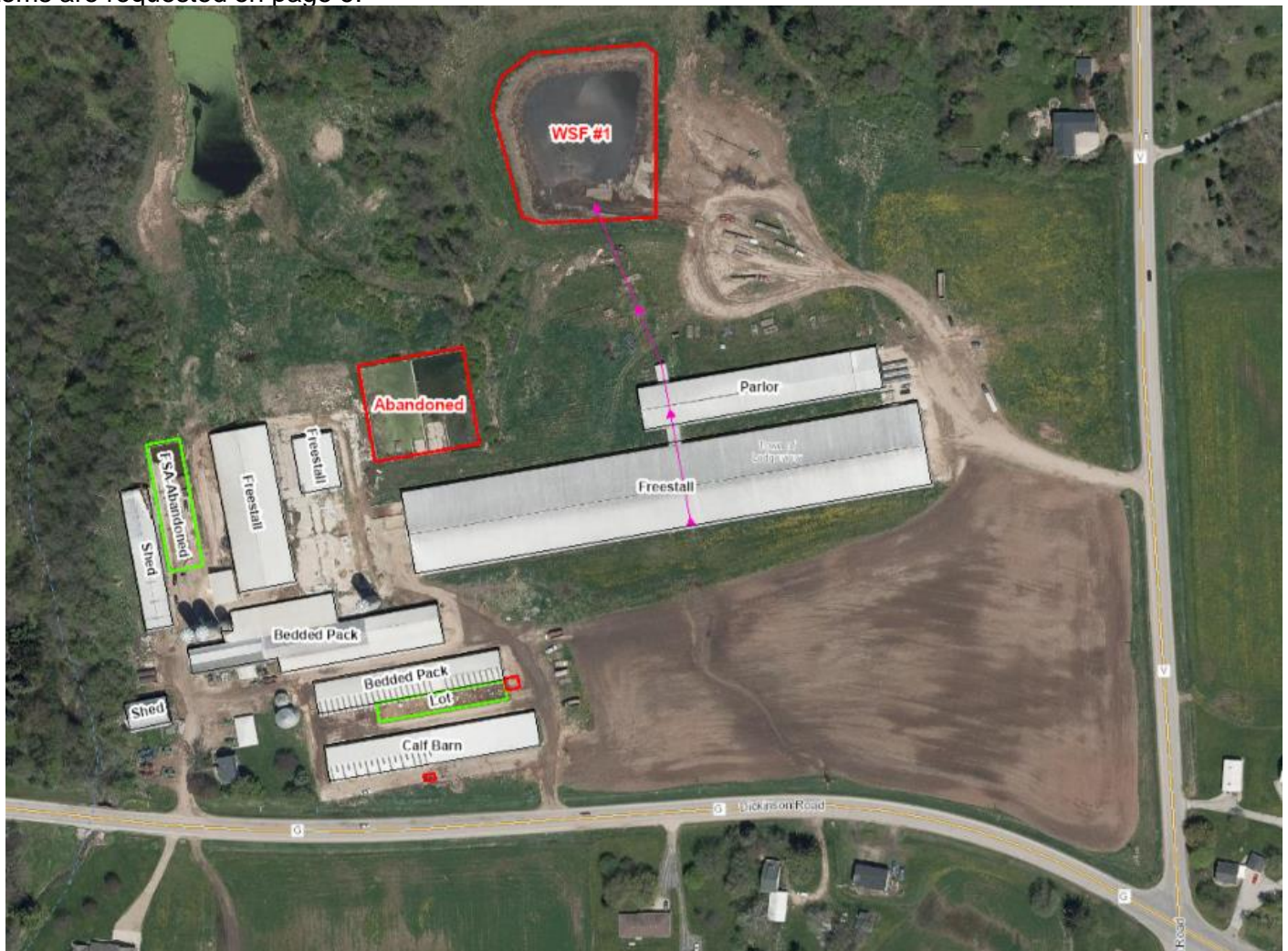
Figure 1. Aerial overview of Ledgeview Farms main site. Approximate contaminated flow paths are indicated with orange arrows. Blue arrows indicate stormwater flow paths. Pink arrows indicate manure transfer lines.
