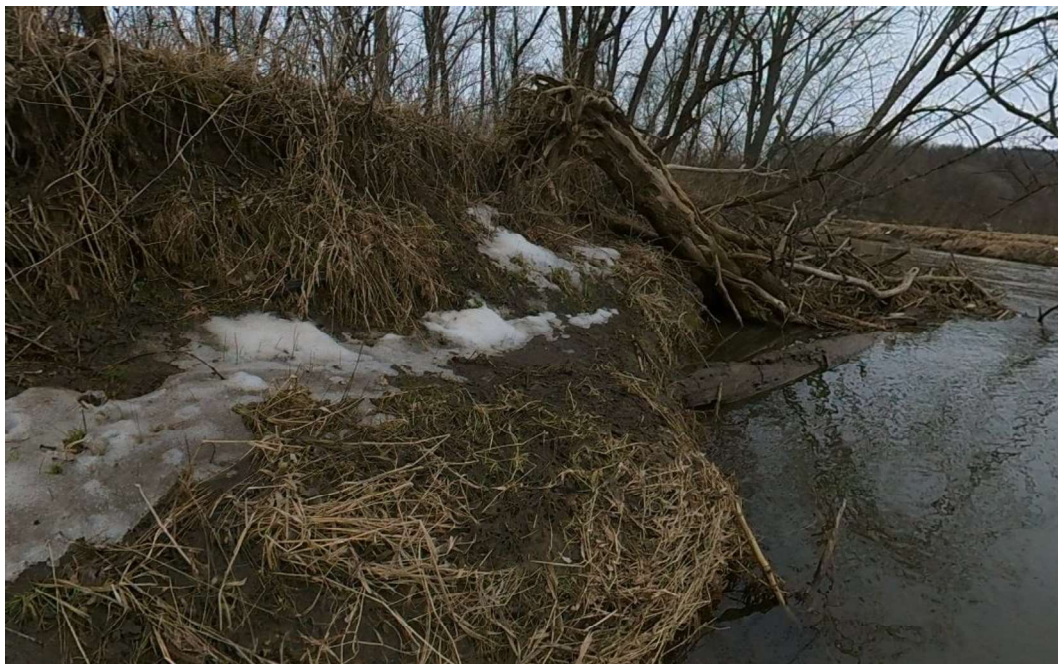
Image 2 – Severe undercut with slump, vegetative overhang, bare soil visible, and fallen trees.
