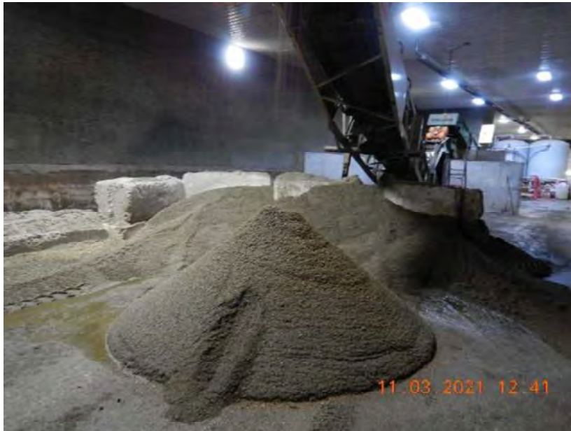
Photo 71. The location where sand is stored at Site 1 until it is reused for bedding in the freestall barns at Site 1. Runoff from the sand piles gravity flows directly to the manure transfer system.
