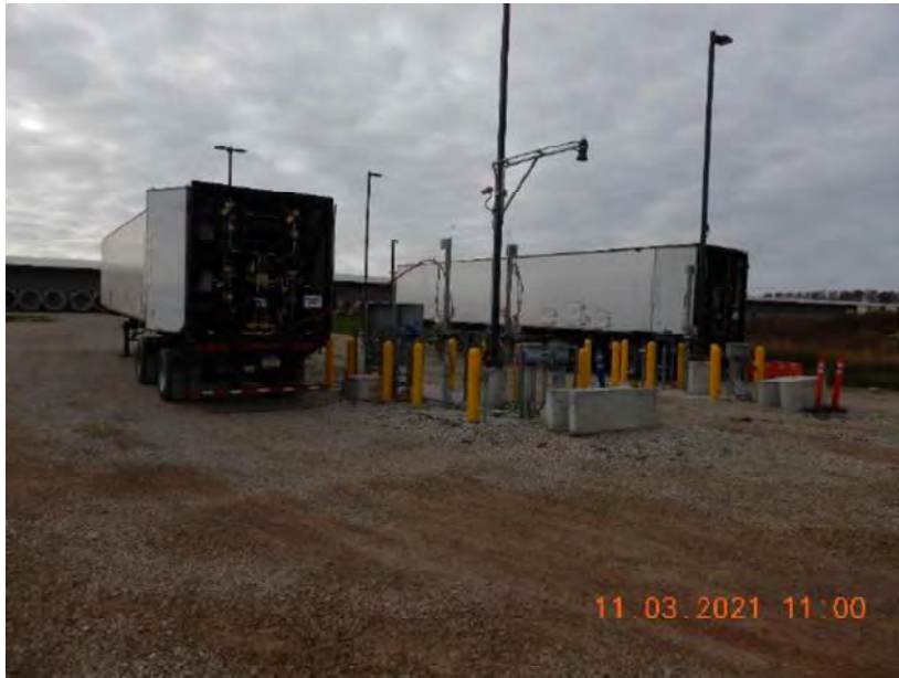
Photo 80. Semi-trailers being loaded with natural gas which will transport the gas off-site.
