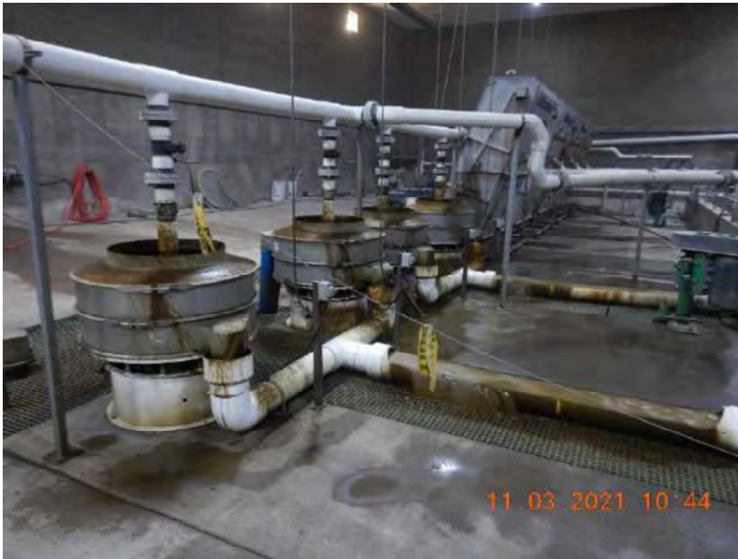
Photo 50. An area where sand is partially removed from manure so that the liquid manure can be flushed back through the manure transfer system and flumes in the freestall barn at Site 2.
