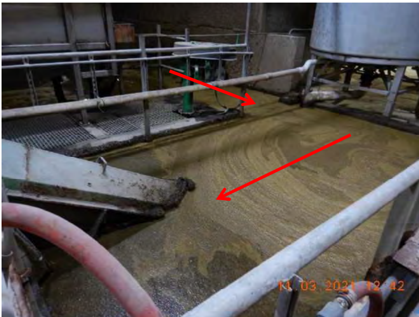
Photo 66. The flow path of manure through the sand separation building at Site 1, represented by the red arrows.
