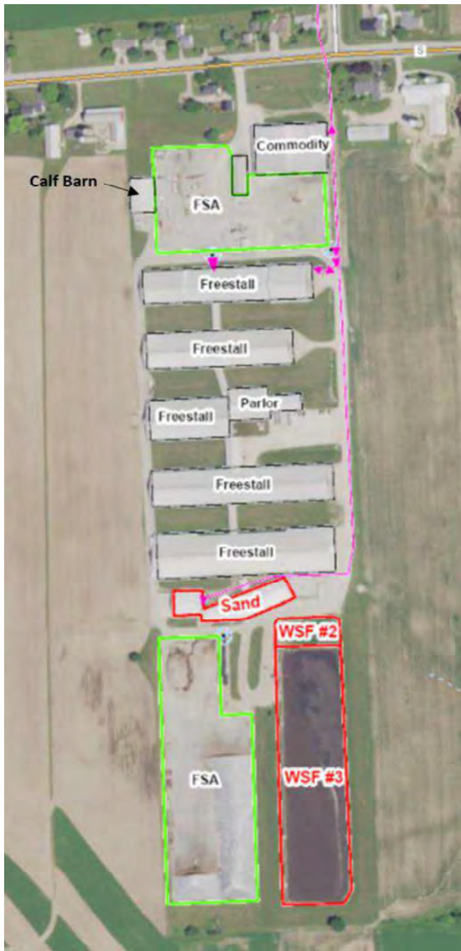
Aerial Map 2. The aerial map above illustrates the production site at Site 1 at Kinnard Farms Inc. Site 1 consists of five freestall barns, one calf barn, one sand separation building, two liquid waste storage facilities, two feed storage areas, and one commodity feed storage building. The pink lines represent manure transfer lines.
