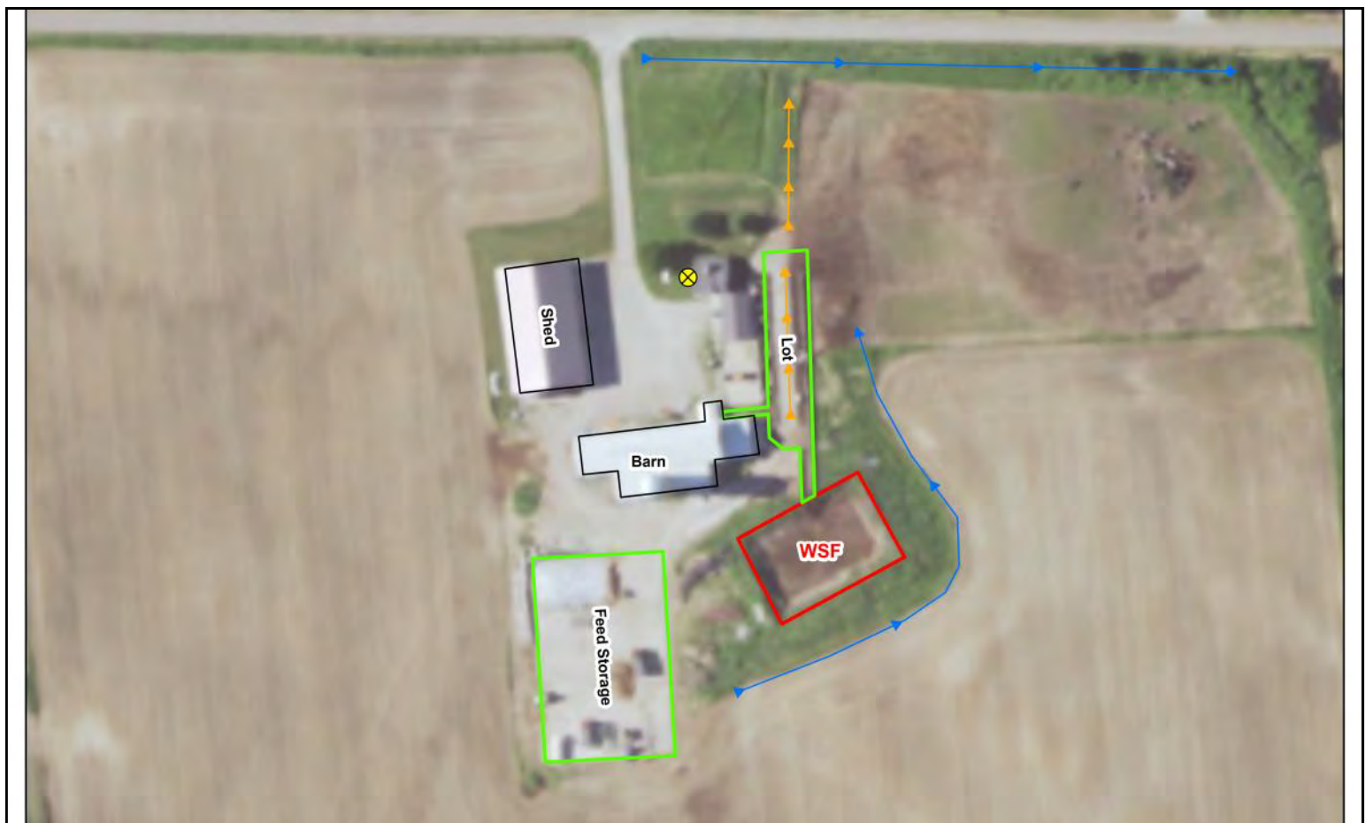
Site Overview Diagram (Heifer Nation LLC: orange lines =potential contaminated runoff, blue lines= stormwater flow, pink lines= waste transfer system, yellow circles = water supply well locations)
