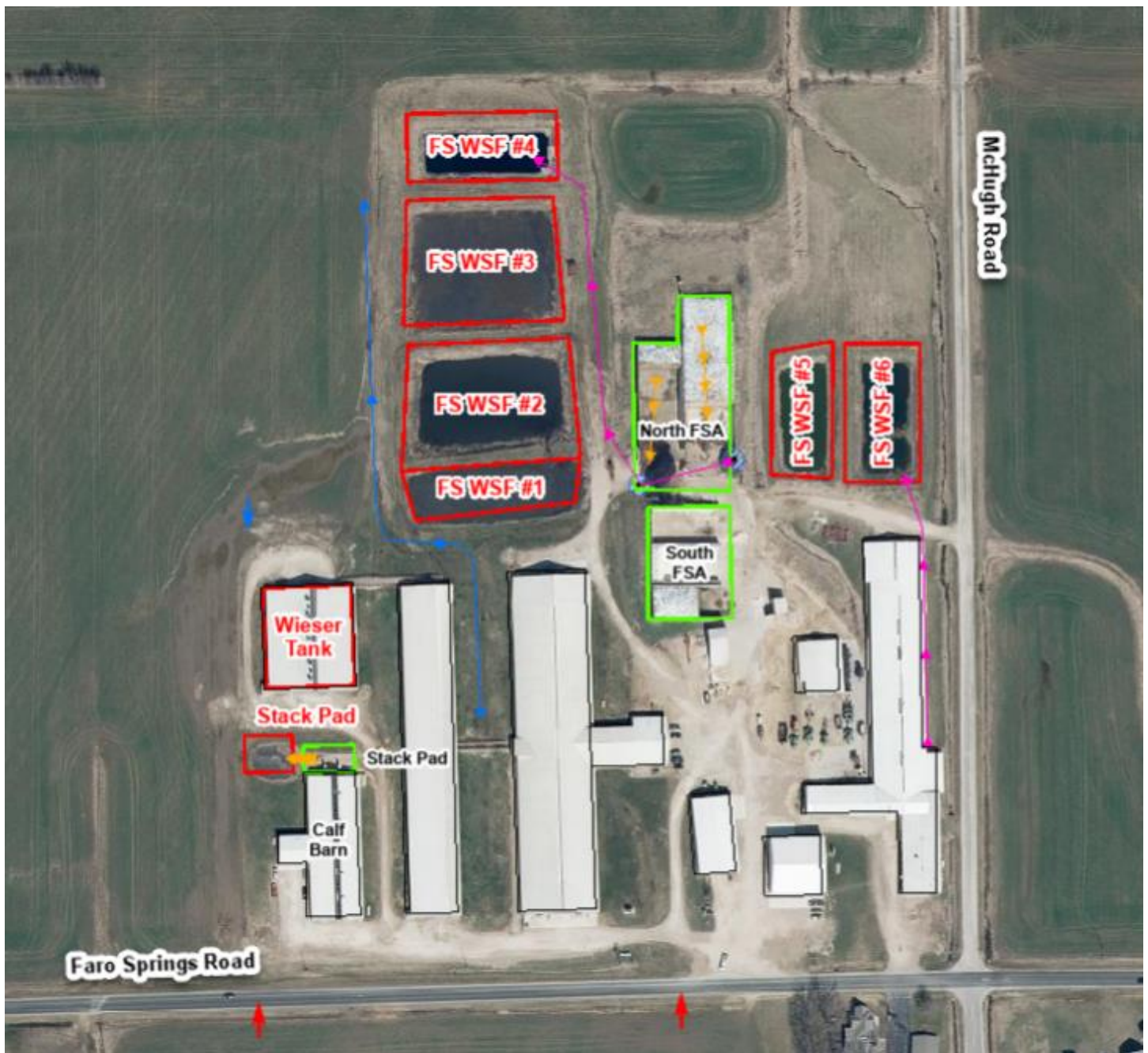
Figure 5. Aerial overview of Holsum Faro Springs. Pink arrows indicate manure transfer lines. Orange arrows indicate approximate contaminated runoff surface flow paths. Blue arrows indicate approximate stormwater flow paths.
