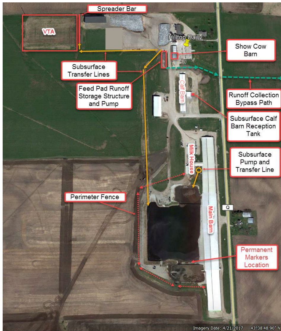
Map 1. Production area map of Hilltop Dairy LLC created by Brenny 2019 Inspection Report
