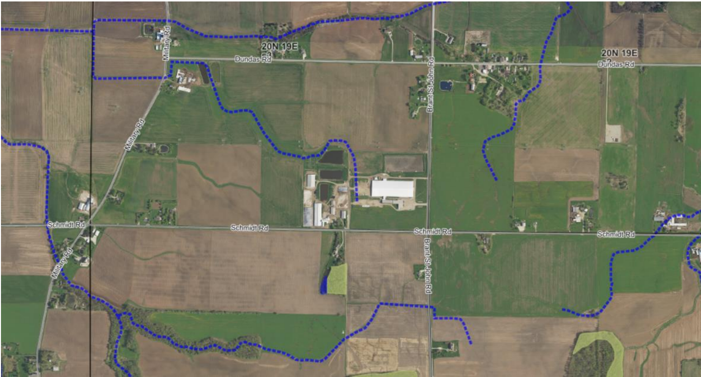
Figure 2. Aerial overview of Grand View Dairy in relation to surface water features. Green areas represent designated wetlands. Dotted blue lines indicate intermittent streams. Image obtained from SNAP Maps v20.
