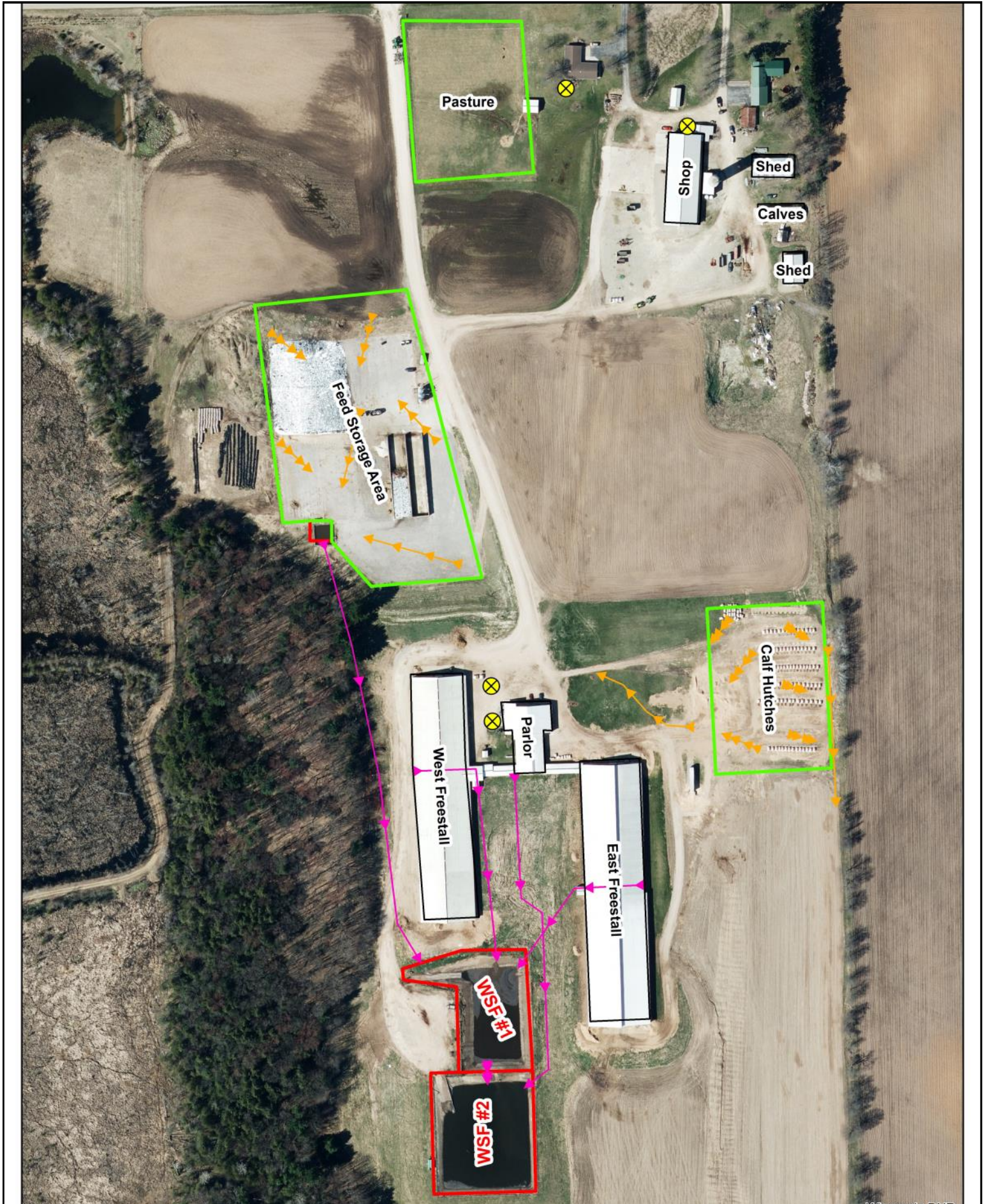
Site Overview Diagram (Golden Ridge Dairy LLC: orange lines =potential contaminated runoff flow paths, blue lines = stormwater flow paths, pink lines = waste transfer system , yellow circles = wells)
