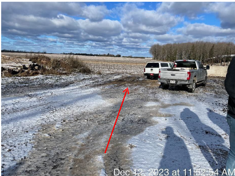
Photo 24. The flow path of runoff from the satellite stacking pad, represented by the red arrows. There are no runoff controls currently in-place.
