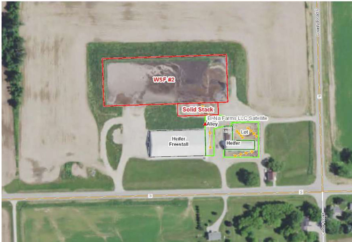
Aerial Map 2. The aerial map above illustrates the production site at the Heifer Site for El Na Farms, LLC. The Heifer Site consists of one liquid waste storage facility, one solid stacking area, one outdoor feedlot, and two heifer barns. The yellow arrows represent the flow path of process wastewater from the feedlots and manure scraping alley.
