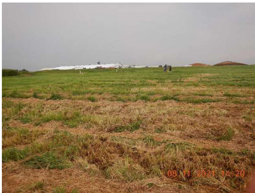
Photo 99. The vegetated treatment area located south of the detention basin. Pictured dead vegetation was killed from excess runoff from one of the bubblers. This photo was taken facing north.
