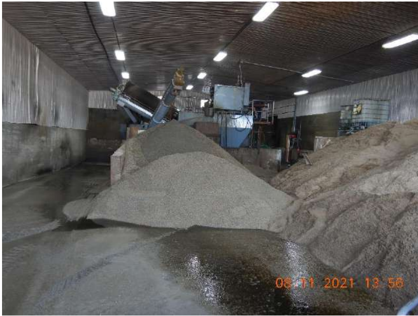
Photo 70. Runoff from the separated sand piles gravity flowing towards a reception basin to be comingled with the manure transfer system and transferred to the on-site waste storage facilities.
