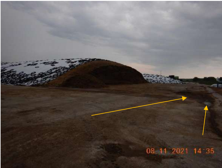
Photo 75. The feed storage area at the Main Site. Runoff flows from north to south and enters one of two runoff control systems. The yellow arrows represent the flow path of runoff. This photo was taken facing north.
