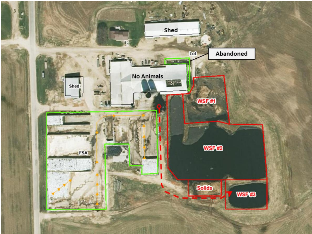
Aerial Map 3. The aerial map above illustrates the east production site at Tonet Dairy. The site consists of a feed storage area, commodity sheds, machine sheds, a solid stacking area, and three liquid waste storage facilities. Animals are no longer housed at the east site.
