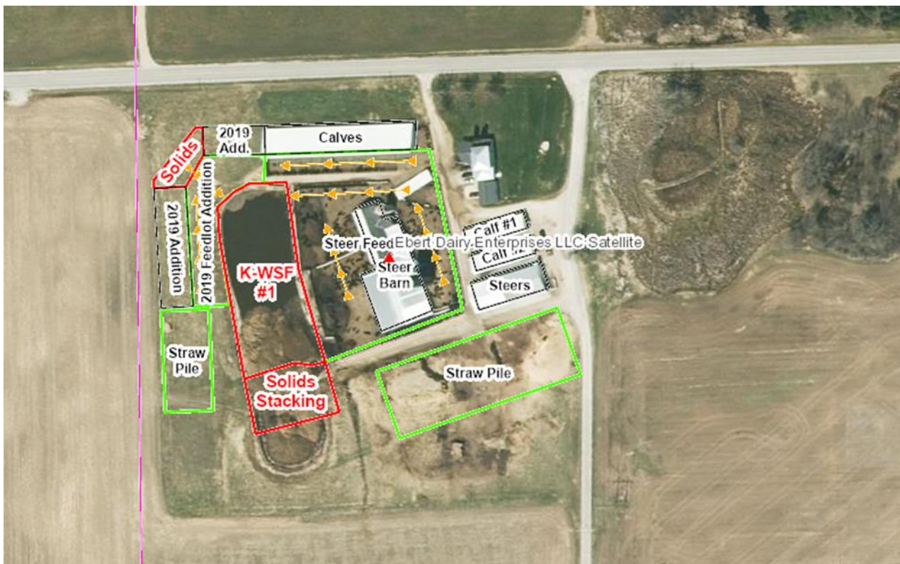
Aerial Map 4. The aerial map above illustrates the production site at the K Farm at Ebert Enterprises LLC. The purple lines represent permanent manure transfer lines. Yellow arrows represent the flow path of process wastewater on the production site.
