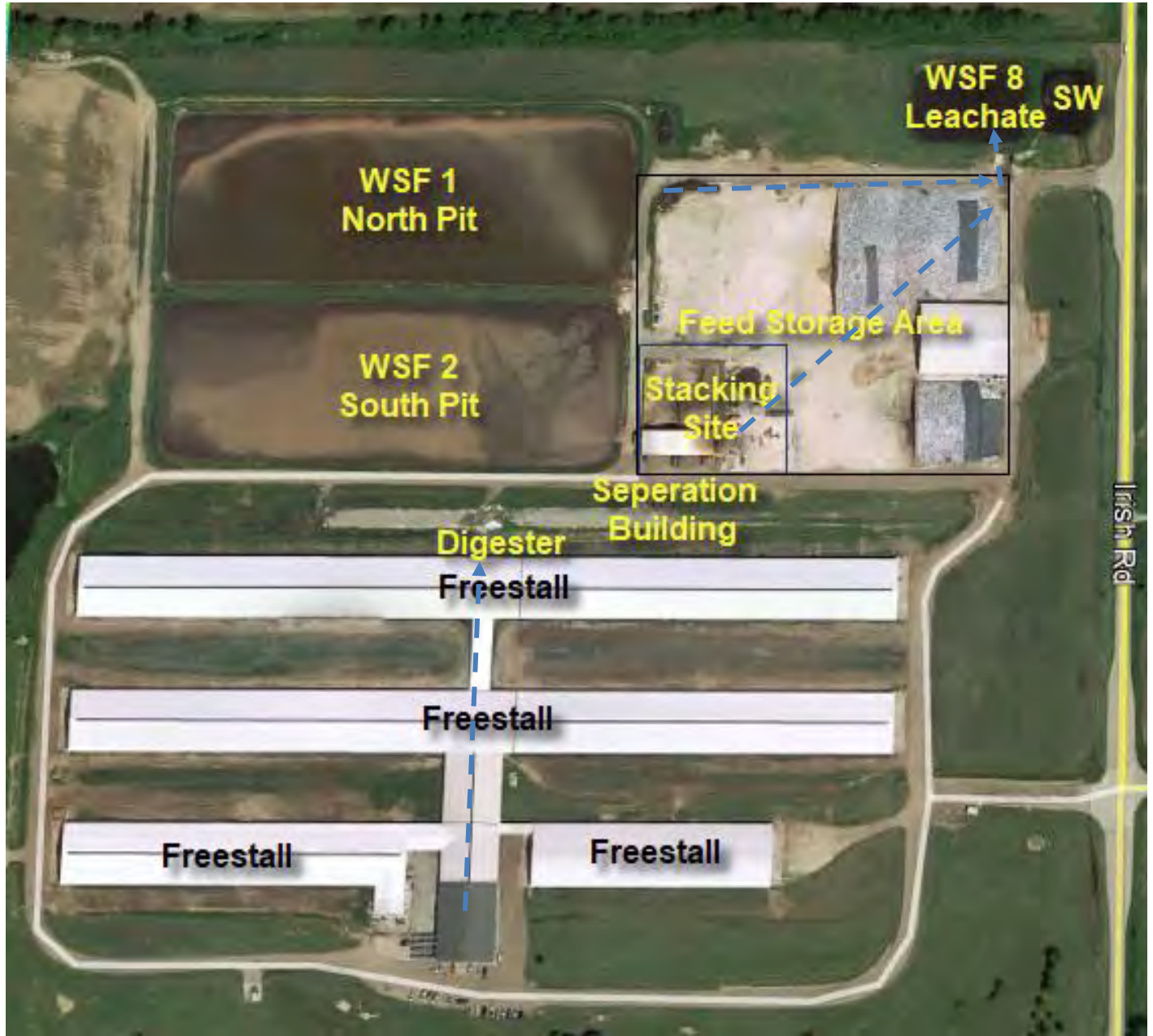
Figure 1. Aerial overview of Holsum Dairy: Holsum Irish Site. Blue arrows indicate flow paths for manure or leachate.
