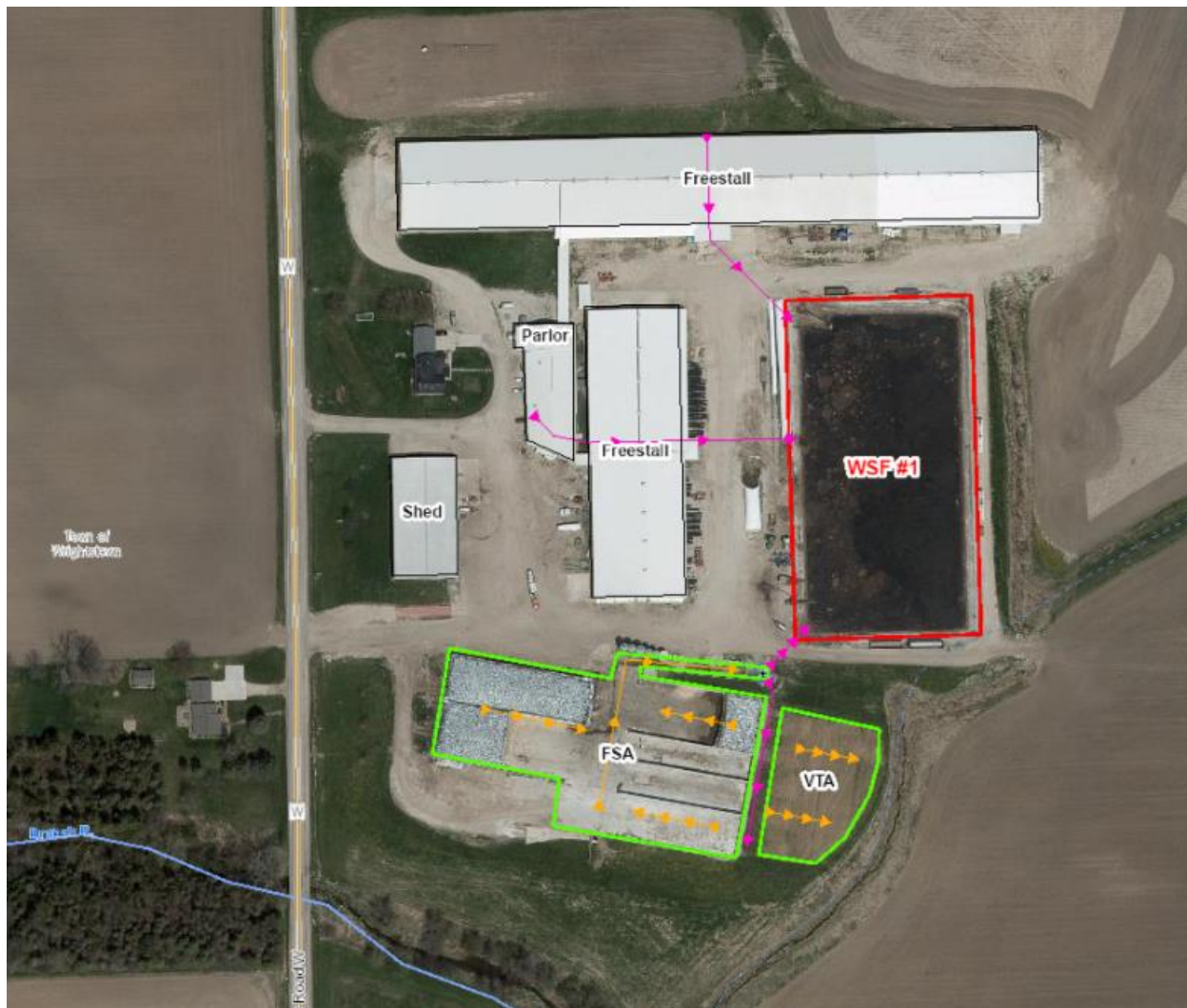
Figure 1. Aerial overview of Denmark Acres. Pink arrows indicate manure transfer lines. Orange arrows indicate approximate contaminated runoff flow paths. Blue lines indicate Branch River. VTA has been abandoned.
