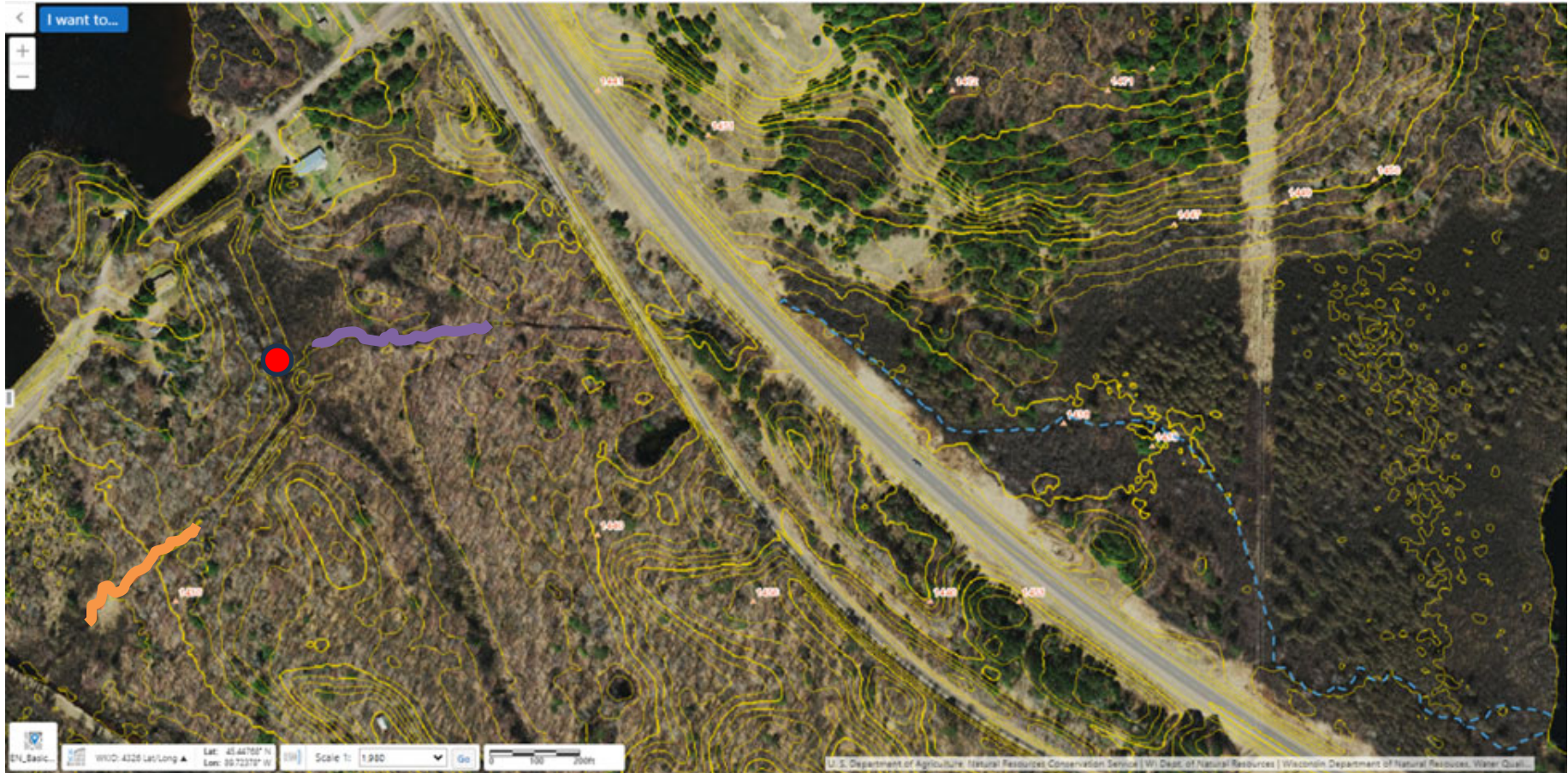
Map 3. Map from Wisconsin Wetland Inventory LIDAR Viewer with derived topography. Fish and Qualitative Habitat Survey Sites/Reaches ( Upstream in purple and Downstream in orange ) as well as outfall location (red circle) are noted. Approximate historic/current probable flowpath from LaCerte Lake to observed CTH S stream crossing noted by hatched blue line.
