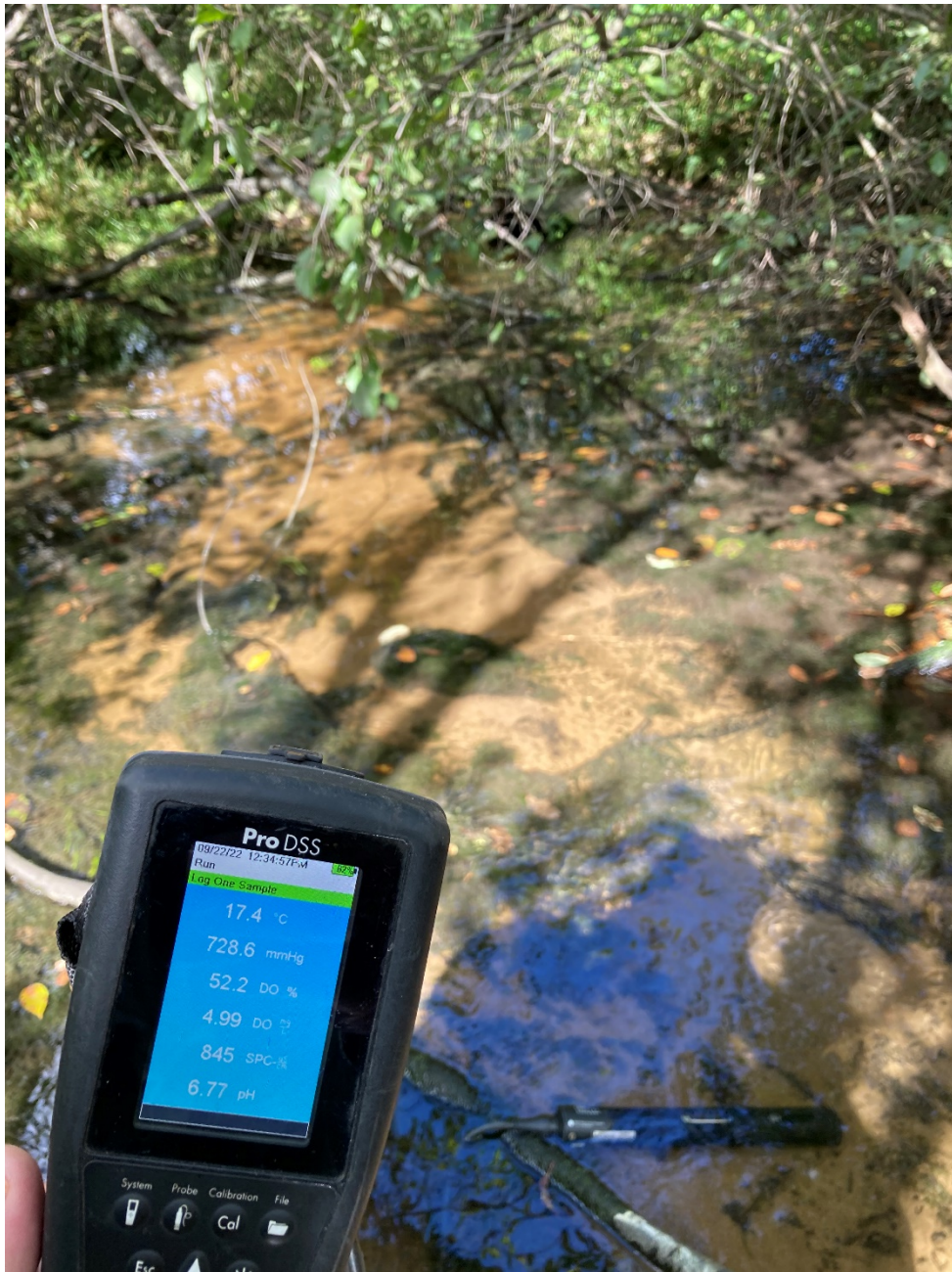
Photo 5. Picture of multiparameter sonde measurements directly downgradient of Tomahawk WWTP Outfall.
