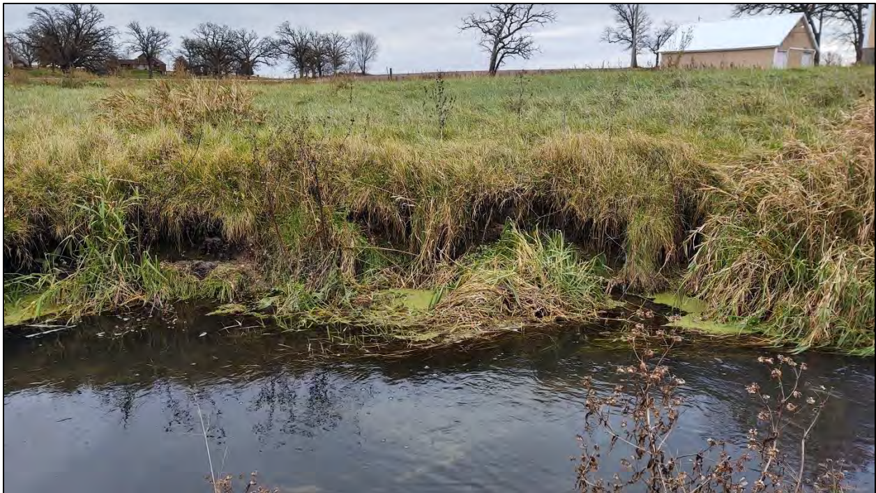
Figure 14: Photograph of new eroding streambank between banks W33 and W34 taken on November 15, 2021
