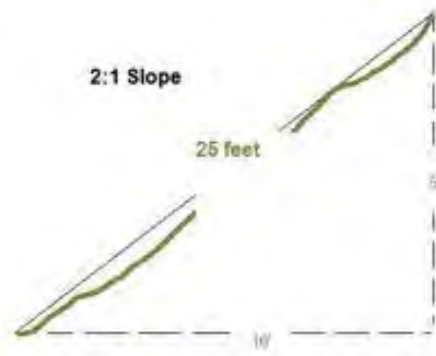
Figure 1: Example measurement of bank slope height. In this example, the bank slope height is 25 ft or the length of the hypotenuse (Source: NRCS Erosion Calculator).
