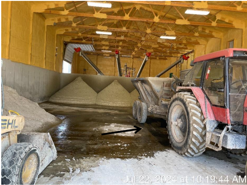
Photo 27. The sand stacking area located in the sand separation building. Leaching from the stacking piles gravity flows to a collection system identified by the black arrow.
