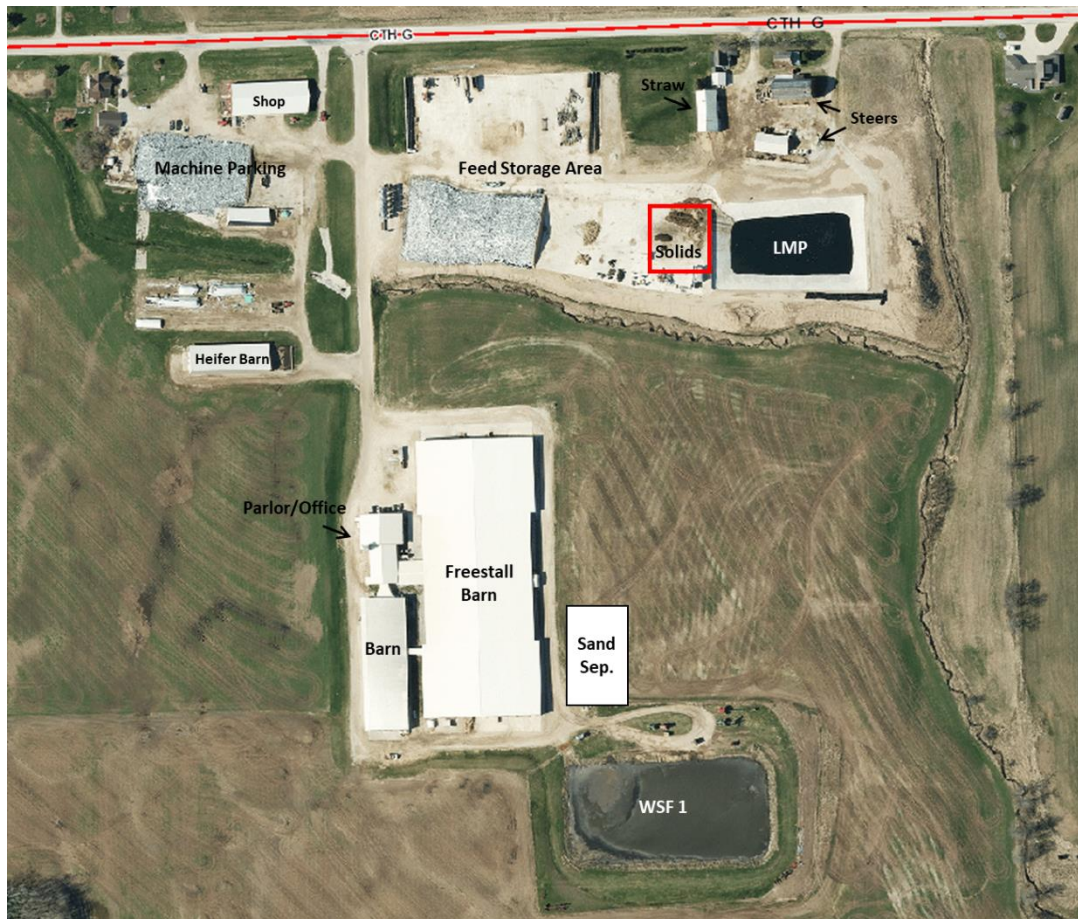
Aerial Map 1. The aerial map above illustrates the production site at Augustian Farms LLC. The production site consists of two liquid storage facilities, one solid stacking area, a sand separation system, several animal barns, and one feed storage area. The aerial image was obtained from Kewaunee County GIS Website.
