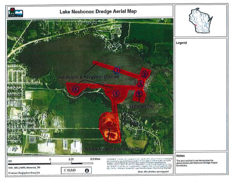
Map 1: shows approximate location of cores to be collected in the proposed dredging area. Proposed core depths are based on maps provided to the Wisconsin DNR (maps 2 and 3 from Cedar Corporation are attached below). If dredging depths vary from the initial maps, core depths should be adjusted accordingly to obtain the entire depth to be removed plus an additional two feet below the dredge depth.
