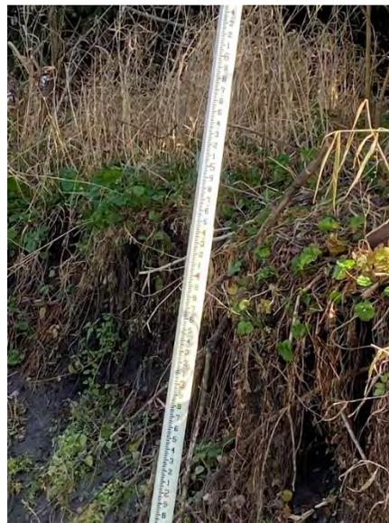
Figure 33.0: Sta. 50+00-50+20 Severe. Bare banks, exposed roots, tree falling into stream, and channel cross-section U-shaped.
