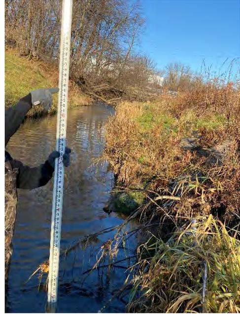
Figure 3.0: Sta. 3+50-6+00 Slight/Moderate. Exposed tree roots, bare banks, and some slumps.
