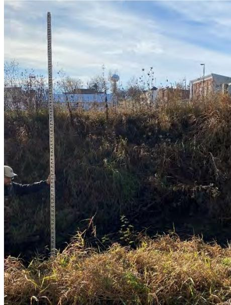
Figure 32.0: Sta. 40+00-40+25 Moderate. Slumps, vegetative overhang, and channel cross-section is U-shaped.
