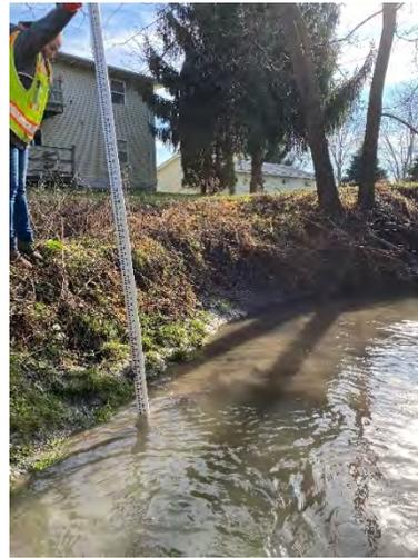
Figure 38.0: Sta. 54+50-55+50 Severe. Bare banks, exposed roots, slumps, and channel cross-section is U-shaped.
