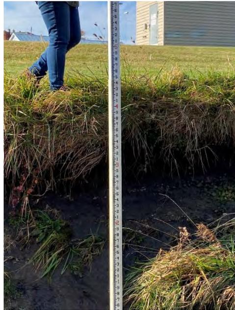
Figure 26.0: Sta. 35+50-36+00 Severe. Bank exposed, channel cross-section U-shaped, slumps/slips, and vegetative overhang.
