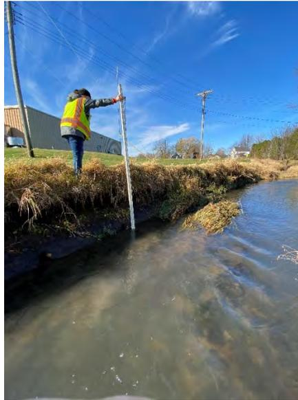
*Figure 28.0 Sta. 36+50-37+50 Severe. Bare banks, vegetative overhang, slumps, exposed roots, and channel cross-section U-Shaped.*
