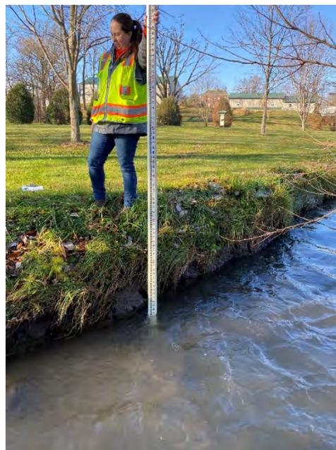
Figure 13.0: Sta. 19+00-22+00 Moderate. Bare banks, vegetative overhang and channel cross section is U-shaped.
