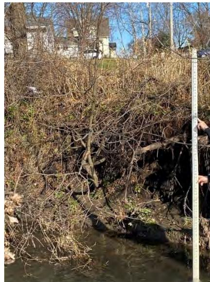
*Figure 29: Sta. 38+75-40+00 Severe. Bare banks, exposed tree roots, trees falling into stream, vegetative overhang, and channel cross-section is U-shaped*
