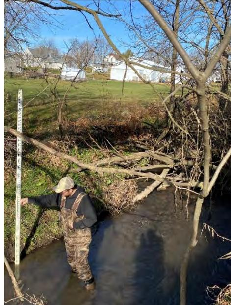
*Figure 34.0: Sta. 50+00-50+20 Moderate. Bare banks, exposed roots and trees falling into stream.*
