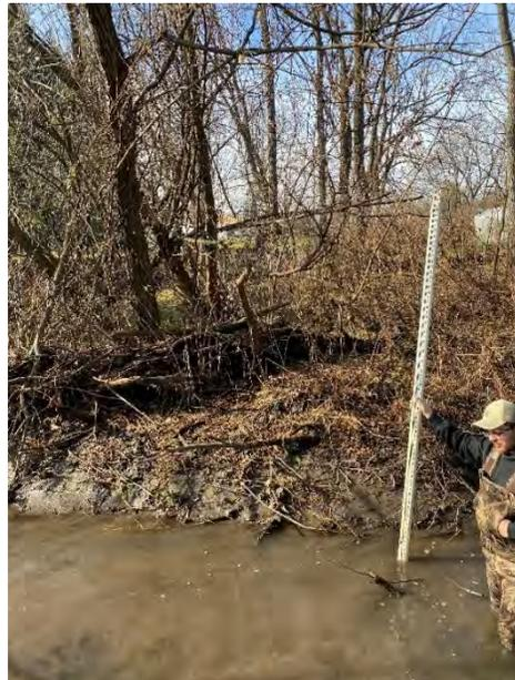
*Figure 41.0: Sta. 56+00-56+50 Slight/Moderate. Bare banks, vegetative overhang, exposed roots, and trees falling into stream.*
