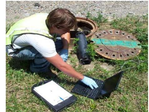
Flow meters are placed at varying locations throughout the collection system. These meters measure the amount and rate of wastewater flow in the sanitary sewer lines. The monitors are left in place for a specified period of time. Data is collected and compared to rainfall amounts over the same period. Measurements taken before and after a rainfall event indicate how much I/I contribute to the total flow of wastewater in the collection system.
