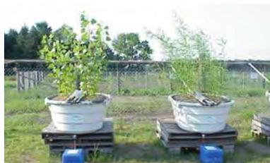
2003: Phases II and III of the treatability study included a tank study and adjacent in-ground planting area. These phases were conducted to refine the design under more representative field conditions and obtain additional performance data on hydraulic uptake and contaminant reduction/removal.
