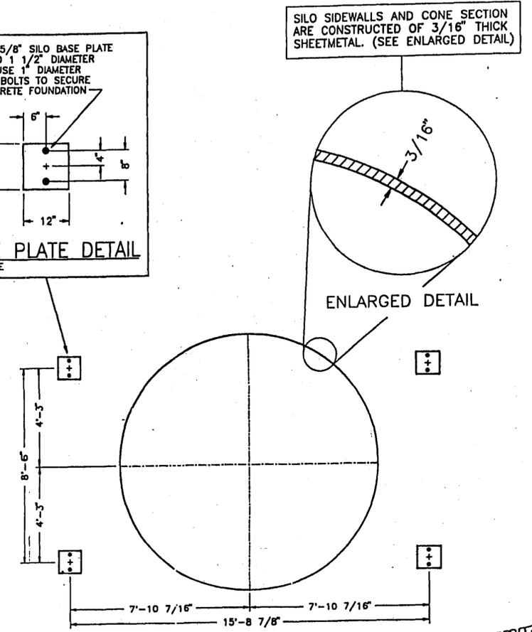
**350 BARREL SILO BASE PLATE AND ANCHOR BOLT LAYOUT**
