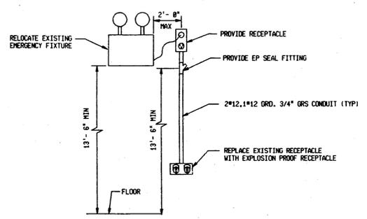
**EMERGENCY FIXTURE MOUNTING DETAIL** (915A)
