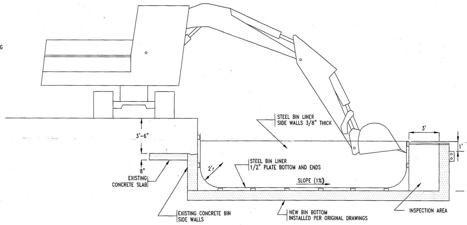
SECTION A-A SHOWING PROPOSED STEEL LINER
