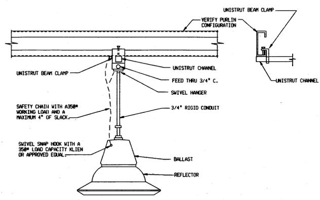
**FIXTURE TYPE "A" MOUNTING DETAIL** (904G)
