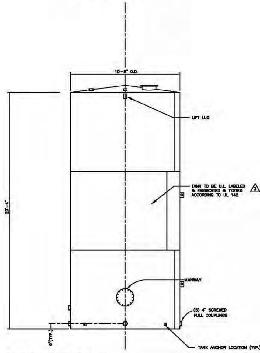
**TANK PLAN AND ELEVATION**
