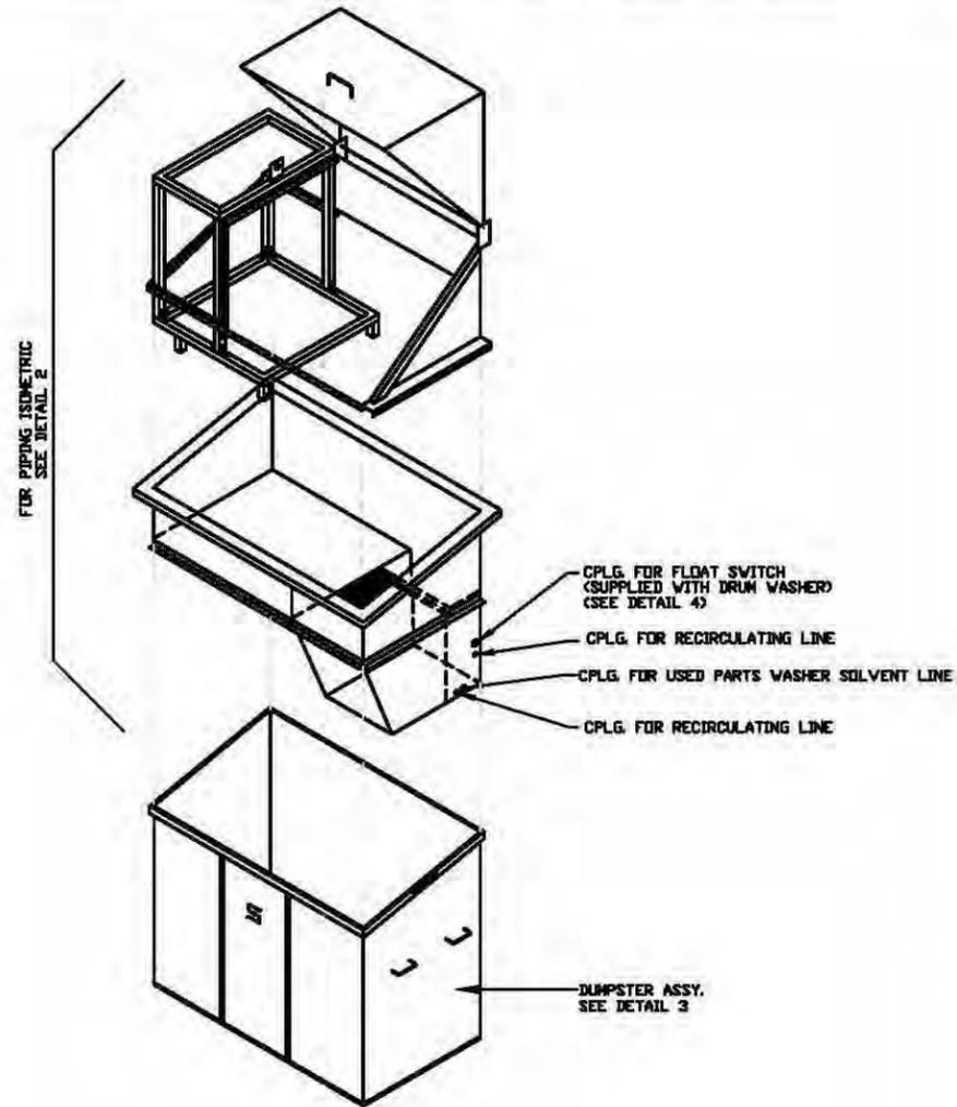
BARREL WASHER PIPING ISOMETRIC - DETAIL 2
