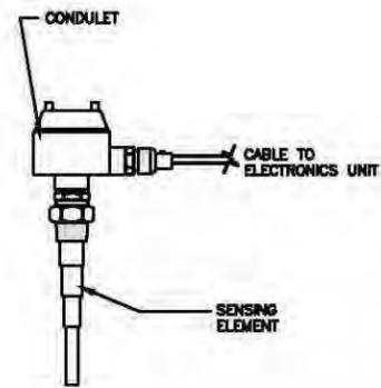
**L.C.T. SENSING ELEMENT AND CONDULET DETAIL**
