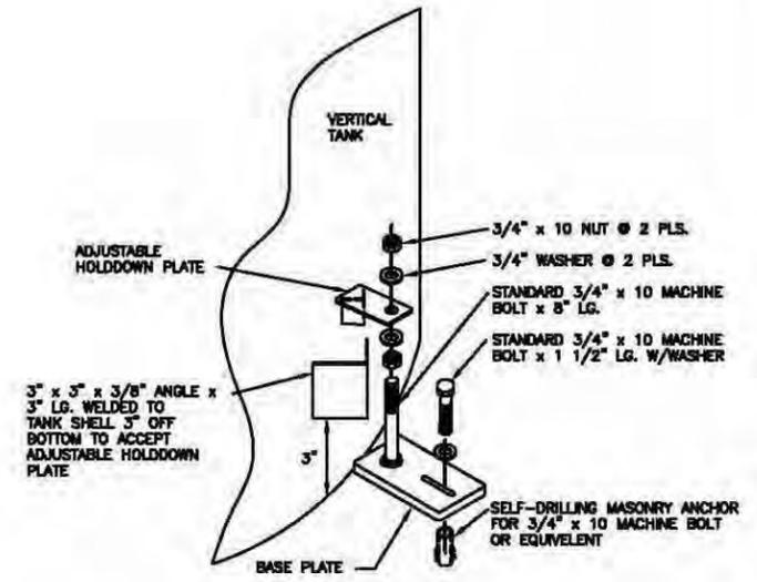
**TANK ANCHORING DETAIL**
