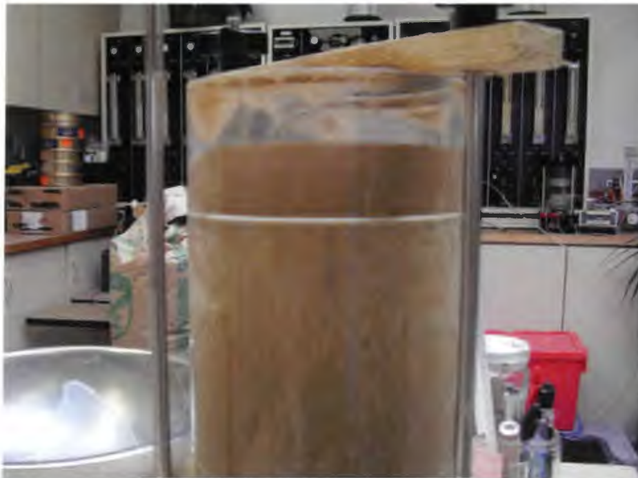
Photograph 6 – The gypsum forms a clear line on top of the coarse sand with no apparent intrusion or migration
