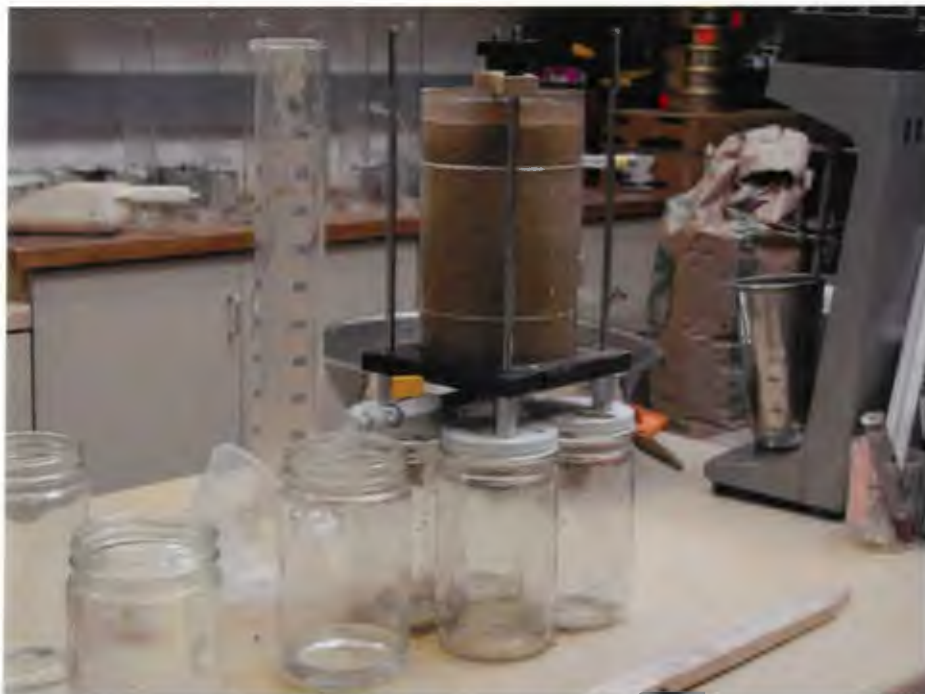
Photograph 4 – The clear filtrate water is collected from the bottom of the apparatus indicating that particulates are not being transported through the sand
