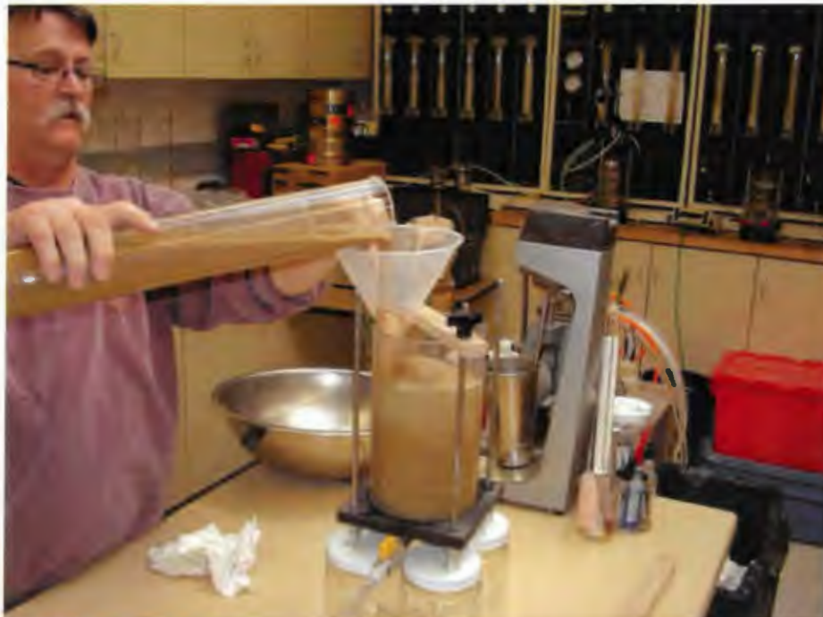
Photograph 2 – The gypsum slurry is poured into the mold on top of the coarse sand the funnel is used to prevent displacement of the sand
