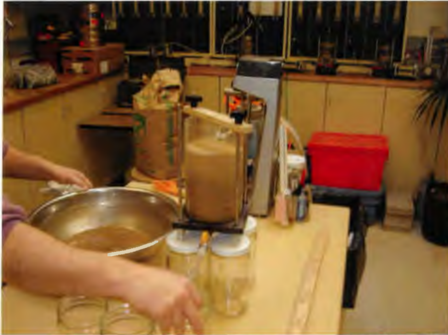
Photograph 1 – Coarse sand is placed in the clear mold and slurry of gypsum and water slurry is prepared
