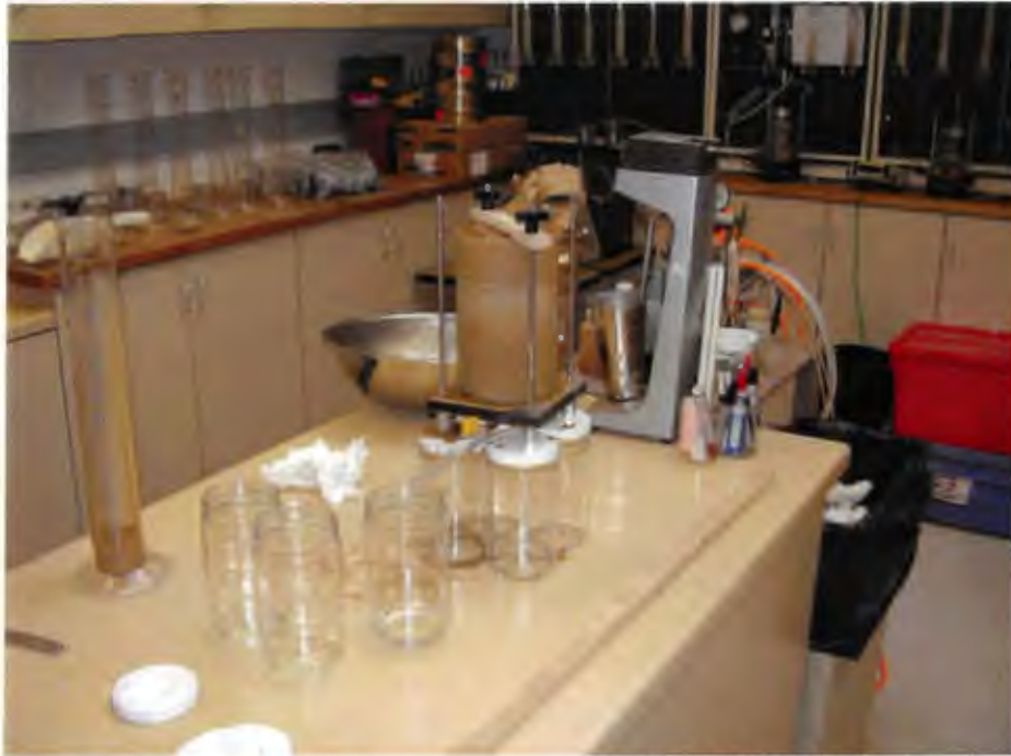
Photograph 3 – The slurry is allowed to drain through the sand and the filtrate water is collected
