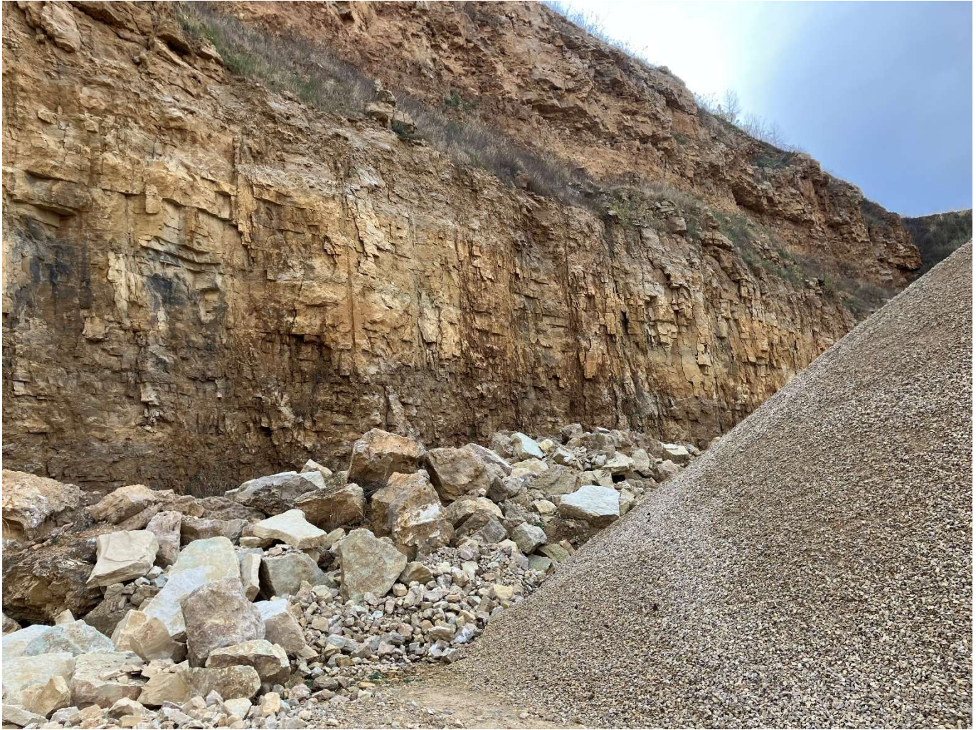
Photo 16 (SEH, October 2025) Gudgeon Pit Quarry – Similar to observations made at Seas Branch Quarry, the shaly layer between the upper and lower bedrock layers within the Hager City Member of the Oneota Dolomite shows evidence of being a pathway for surface water percolating downward through the unsaturated bedrock; these pathways in the unsaturated bedrock layer may locally intersect the quarry wall and seasonally form seeps. See Photo 14 for more descriptive details.
