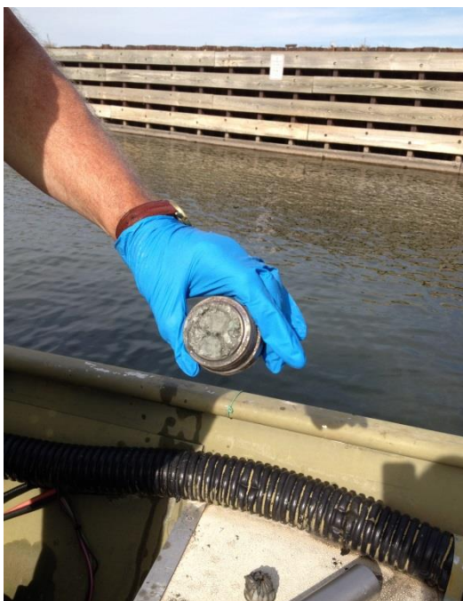
Photo 13. Sediment Sample, Firm Clay at Sample Location A-1 (Lower Sample A-1.2)
