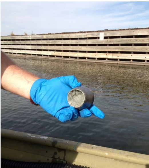
Photo 14. Sediment Sample, Firm Clay at Sample Location A-1 (Lower Sample A-1.2)
