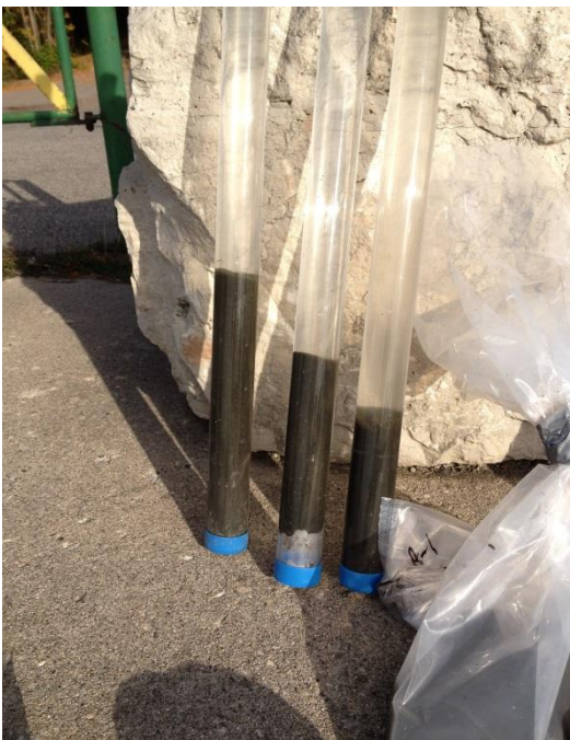
Photo 15. Sediment Samples in Butyrate Tubes
