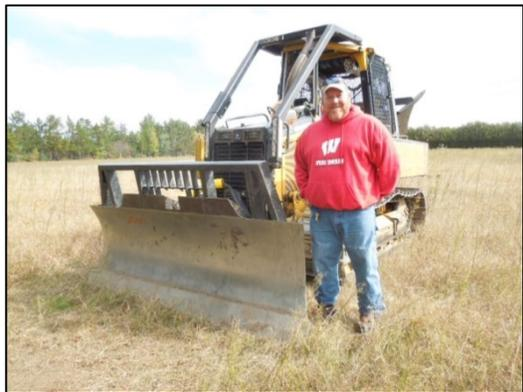
before harvest to expose mineral soil and promote seed germination. When operating post harvest, stumps need to be low to prevent bumping or hanging up on the stump. The straight blade can be mounted on various sizes of bulldozers and are widely available.
