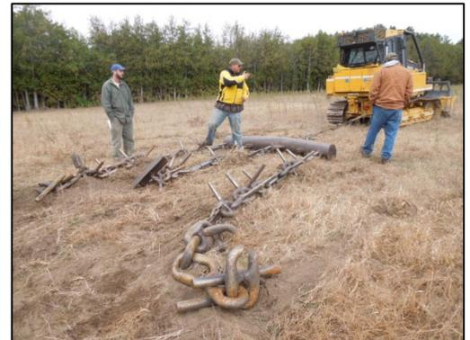
**Root Rake** – A root rake operation is preferably done when the ground is frozen and snow depth is less than two feet, or from mid-summer to early fall if the soil is dry. It is best suited for well-drained soils as those with a clay component are susceptible to compaction, especially when wet. This equipment is used to perform light scarification for seeding and to pile
