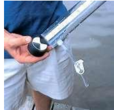
Figure 10. Secchi symbol at the bottom of the transparency tube.
