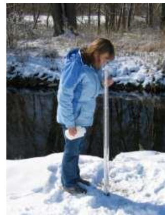
Figure 1: Transparency tube shaded by observer
