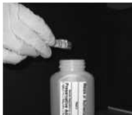
Figure 2. Add a vial of sulfuric acid to sample. Be sure to place cap topside down to avoid contamination.
