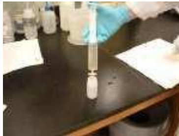
Figure 8. Hold filter over 60 ml bottle and press plunger down slowly.
