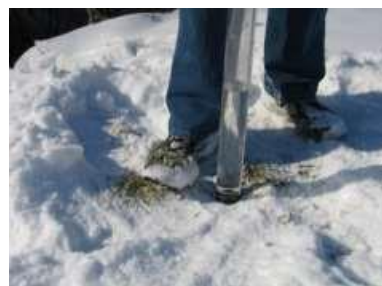
Figure 12. Slowly releasing water until the disc is just visible.
