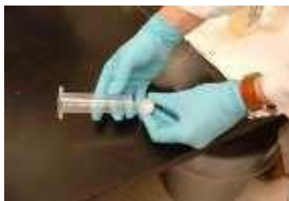
Figure 6. Screw the filter onto the syringe tip.
