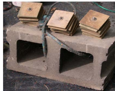
River Macroinvertebrate Hester-Dendy Sampling Device
