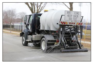
weather conditions or applying Brine that is not the correct formula can be disastrous. Brine shall be made by a select few in the department who are trained on the Brine making machine. The Brine making machine shall be cleaned for every 30,000 gallons of Brine made.
