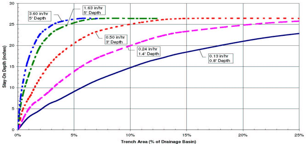
Note: The 5 ft. depth depicted in the Infiltration Trench Design Curves chart is not a limitation to the depth of an infiltration trench.
