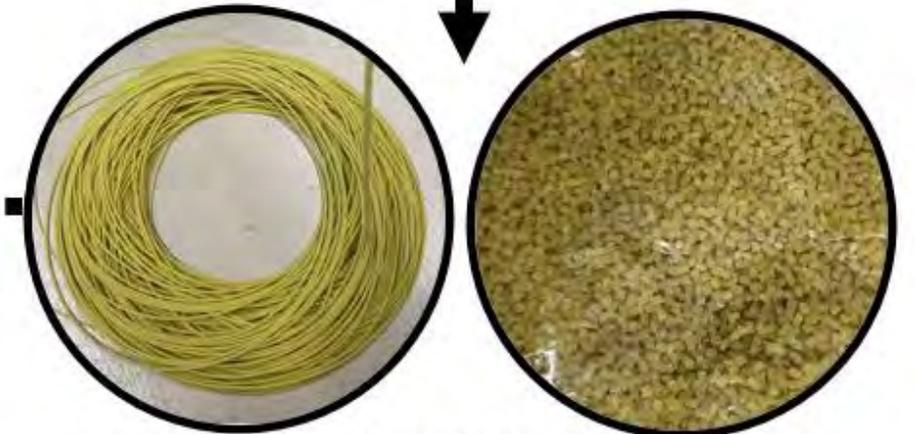
**Extrusion and pelletization of the recovered PE**
