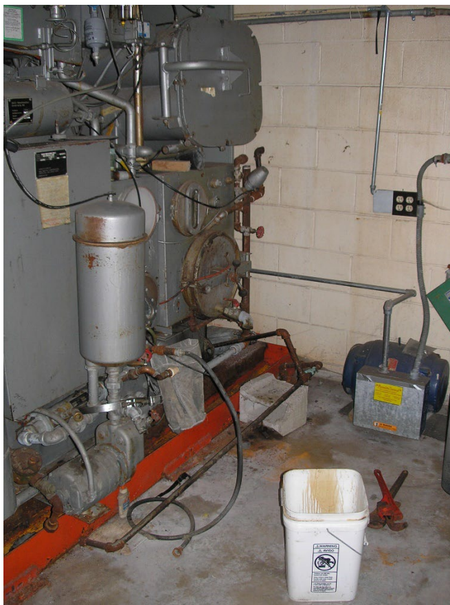
Photo 4. Back of dry cleaner machine where spent filters were rinsed out directly onto the floor for filter reuse as reported by the operator. Wastewater was left to seep into floor cracks, open cinder block wall or evaporate.
