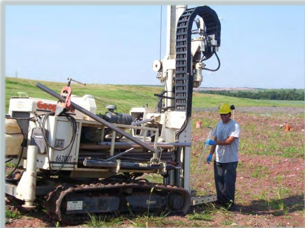
Example of direct push sampling for soil and groundwater
