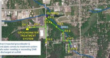
9 wells extract impacted groundwater & underground pipes convey to treatment system on FTC. Safe water meeting or exceeding DNR standards discharged at outfall.
