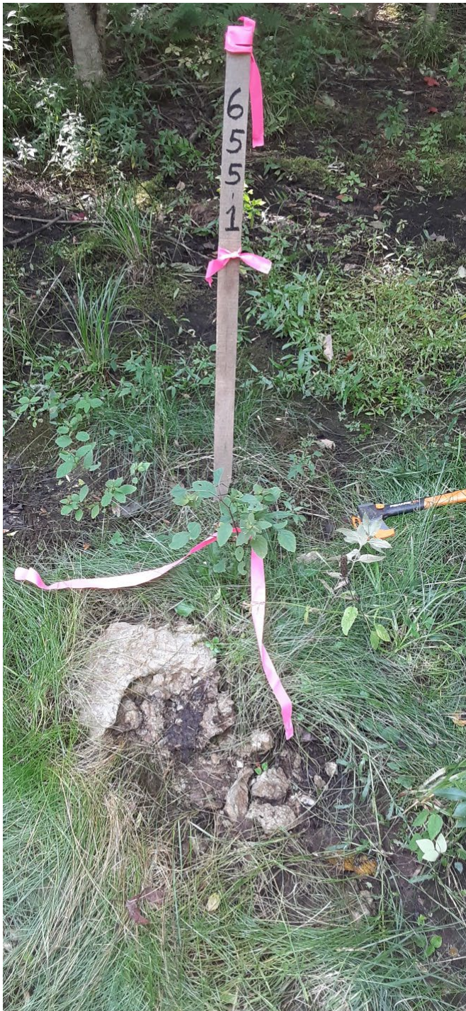
Photo 4: Close up view of grout cap at Exploration Hole 655-1.
