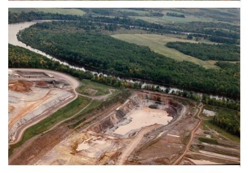
Aerial view of the Flambeau Mine shows the pit with accumulated precipitation and groundwater in the bottom and its close proximity to the Flambeau River. To the left is the high-sulfur waste rock stockpile, ore crushing area, rail spur, and an engineered runoff pond (Photo by Bob Olsgard of Sarona, WI, September 17, 1994).
