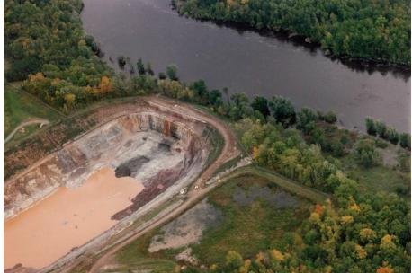
FMC's water treatment plant couldn't keep up with all the rainwater and groundwater that poured into the mine pit. Four feet of water accumulated in the bottom, totaling about four million gallons according to FMC estimates (Photo by Bob Olsgard of Sarona, WI, September 17, 1994).
