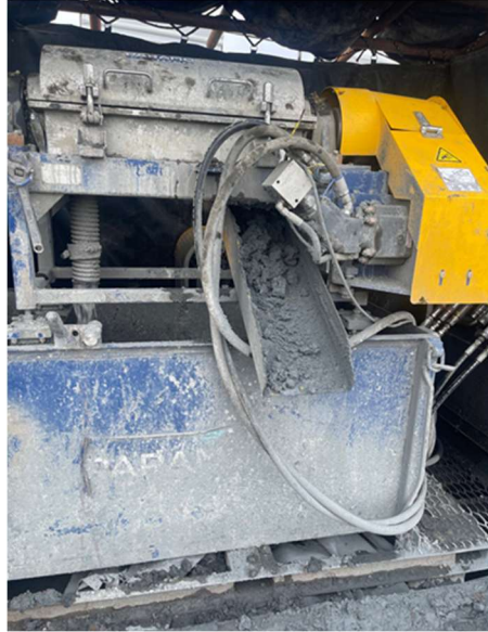
Figure 5 – Image of removed cuttings using a solids removal unit (centrifuge)
