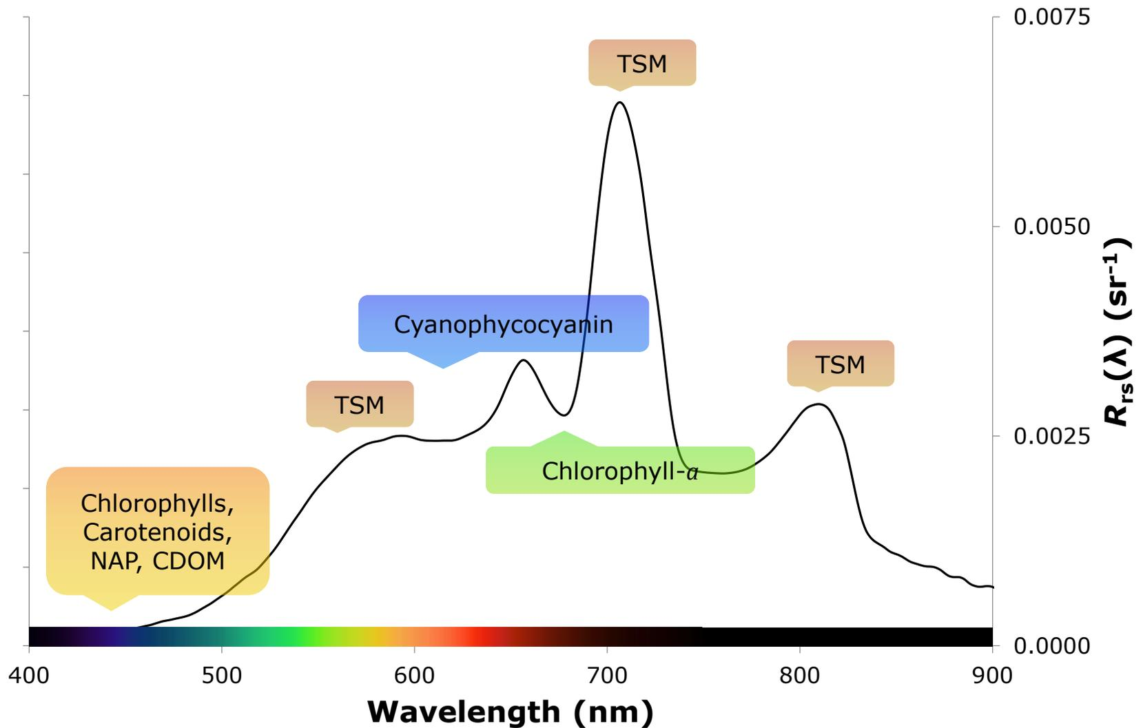
Remote sensing reflectance spectrum for the Spirit River Flowage acquired on 07/21/2015. This remote sensing reflectance spectrum is typical for some of the stained lakes and their high concentrations of CDOM in northern Wisconsin (NAP – non-algal particles, CDOM – colored dissolved organic matter, and TSM – total suspended matter).
