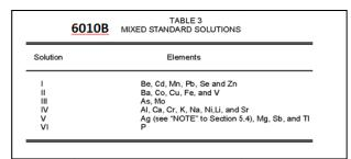
If verifying lack of interference is difficult when analyzing a single standard containing all elements, how could that possibly work for calibration? It doesn't. And the two methods suggest different groupings of standards because each of the methods recommends different analytes and wavelengths.
