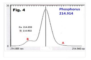
Figure 5A seems, at first glance like a no-brainer. Either side looks clear (from the single element standard view!). While either side of the target peaks appears to be appropriate for background correction (based on this scan), a decision is made to make background correction on the longer wavelength side. And that's why we have to consider what else COULD appear (and impact background correction).
