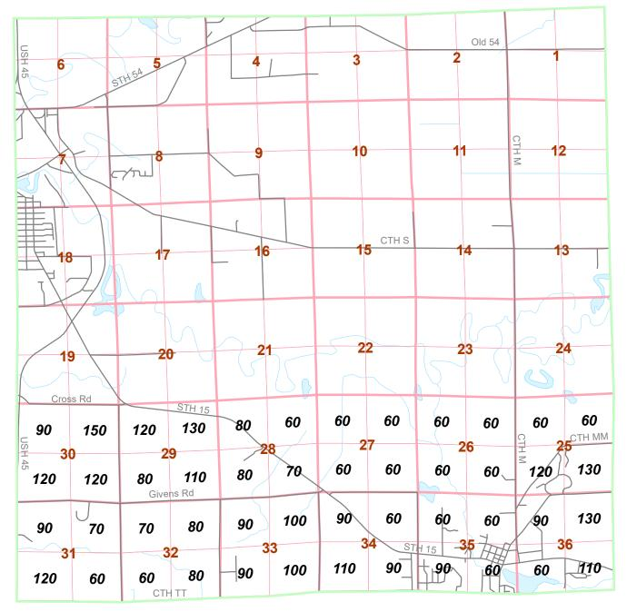
\*Within each quarter section the minimum depth of the upper-enlarged drillhole, casing pipe, and cement grout is indicated by the number provided. Although unlikely, the minimum casing/grout depths provided above may not get you down to the Cambrian Sandstone. However, in any case, the casing and grout shall extend at least to the top of the Cambrian Sandstone.
