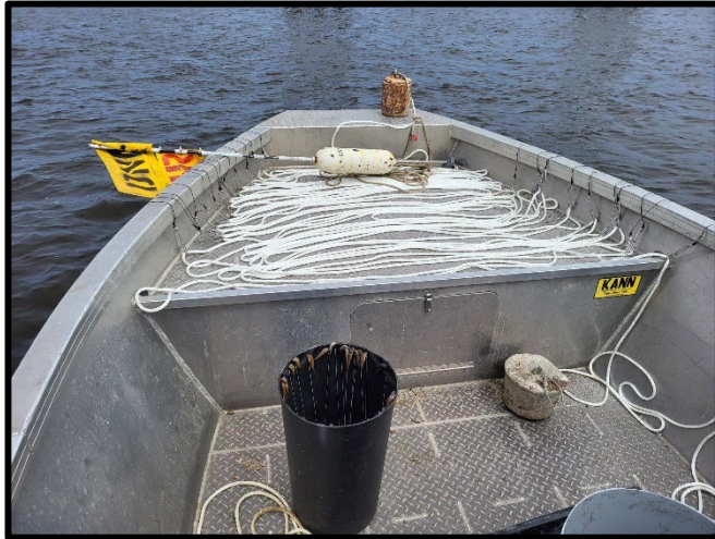
Image 8. A set line rigged on the front of the DNR boat immediately before setting.
